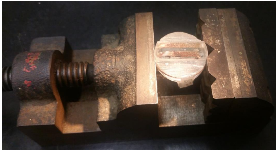
Figure 3.1 Trabecular Bone Sample Secured in Vice with V-block Insert
